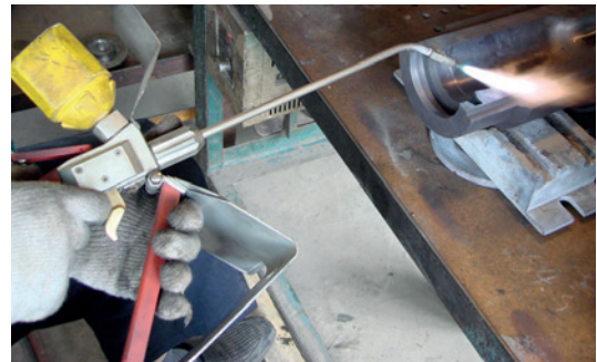
Figure 16 Powder welding of mould edge
