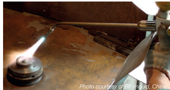
Figure 19 Thin layers minimise oxidation
